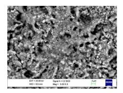
Fig.1. Back-scattered electron image of the surface the TiO<sub>2</sub>-2.5vol.%Ag coating formed by detonation spraying at an explosive charge of 60% and  $O_2/C_2H_2 = 1.05$ .
