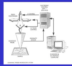
In each "point", measure of a "local" physical quantity related with the interaction: in STM the tunneling current, in AFM the cantilever deflection, due to attractive or repulsive force.
