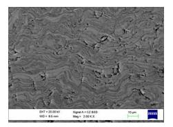
Fig.2. Back-scattered electron image of the microstructure of the coating formed by detonation spraying of  $Ti_3AI$  at an explosive charge of 50% and  $O_2/C_2H_2$  =1.50.
